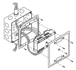
SIGA-MCC1 and SIGA-MCC2: mount the UIO motherboard inside a suitable GE Security enclosure with screws and washers provided. Plug the SIGA-MCC1 or SIGA-MCC2 into any available position on the motherboard and secure the module to the motherboard with the captive screws. Wiring connections are made to the terminals on the motherboard (see wiring diagram). UIO motherboard terminals are suited for #12 to #18 AWG (2.5 mm² to 0.75 mm²) wire size.
