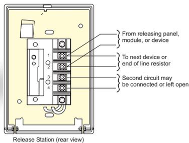
The manual release station is a normally-open, dry contact signal initiating device. The 276A-REL is a single-action station that requires the user to pull the release handle to initiate the release of a fire suppression agent. The 278A-REL (shown) is a double-action station that requires the user to raise the upper door, then pull the release handle to initiate the release.
